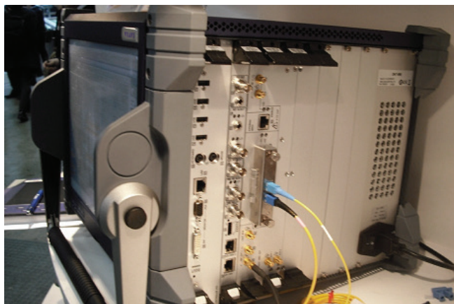
Figure 5. CFP LR4 module inserted in ONT tester
